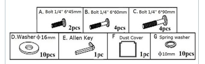
**STEP1** Attach the Seat(3) to the Back frame (1) with Bolt(C), washer(D) and Spring washer (G) using Allen Key(E).
